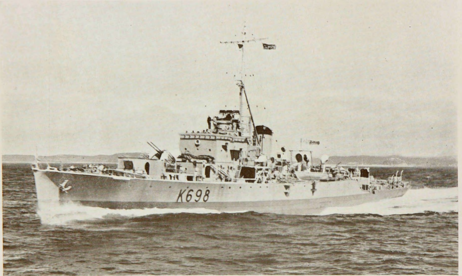
H.M.A.S. "CONDAMINE" — TWIN SCREW RIVER CLASS FRIGATE. 307 Ft. long; 5,500 I.H.P.; Speed 20 knots; — undergoing Trials.
