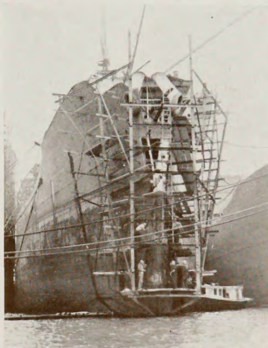
VIEWS ILLUSTRATING DAMAGE AND HOW REPAIRS WERE EFFECTED UTILISING STEEL SCAFFOLDING WELDED TO HULL.
